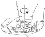
Undo the screw in the centre of the pulley and remove the pulley. Insert and fasten a new starter cord to the pulley. Wind approx. 3 turns of the starter cord onto the pulley. Connect the pulley to the recoil spring so that the end of the spring engages in the pulley. Fit the
