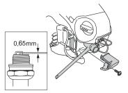
Note! Always use the recommended spark plug type! Use of the wrong spark plug can damage the piston/cylinder. Check that the spark plug is fitted with a suppressor.
